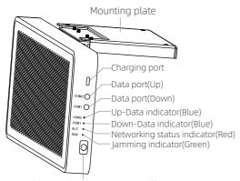
Control button (press to turn on/off jamming, press and hold 3S to restore factory settings)
